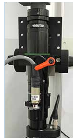
Optotune Module (Navitar 1-64805) with Zoom 6000 Motorized System
